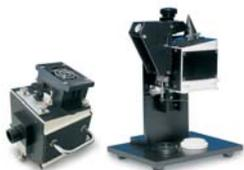
**Reflectance attachment with spectralon integrating sphere**
