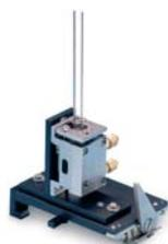
**Thermostated and adjustable HPLC cell holder**
