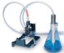
**Fiber coupling with transmission immersion probes and HELMA fiber adapter**
